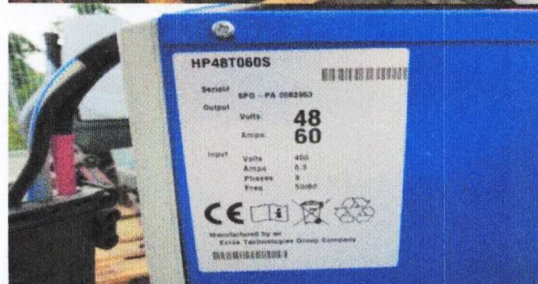
Fot. 30-31. Prostownik model HP48T060S
